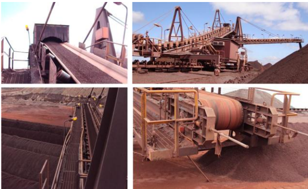
Figure 10: Tripper with Stacker (top right), Transfer Point Tripper to Stacker for Volume Flow Measurement (top left), Boom with Windrow Cones in background (bottom left), Stacker boom head idler pulley (bottom right)
