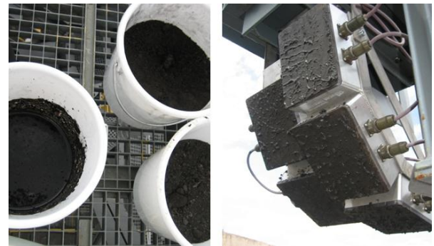
Figure 8: Radar blockage test with mixture of clay, sand and coal
